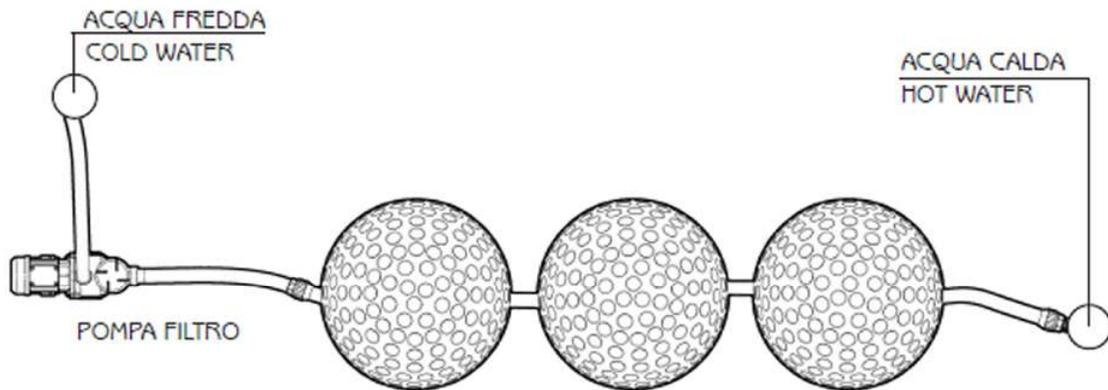
Sistema montato in parallelo / Parallel fixing system
